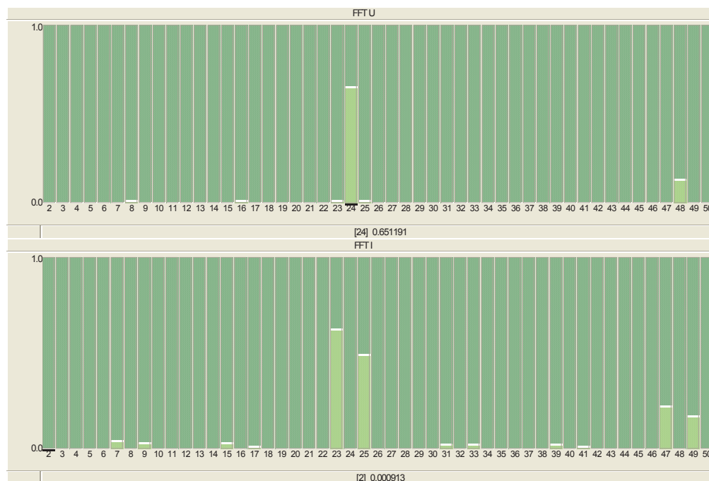
Figure 3-17 FFT analysis for Harmonics** Superposed alternating voltage on the DC side (above) harmonic current on the AC side (below)
