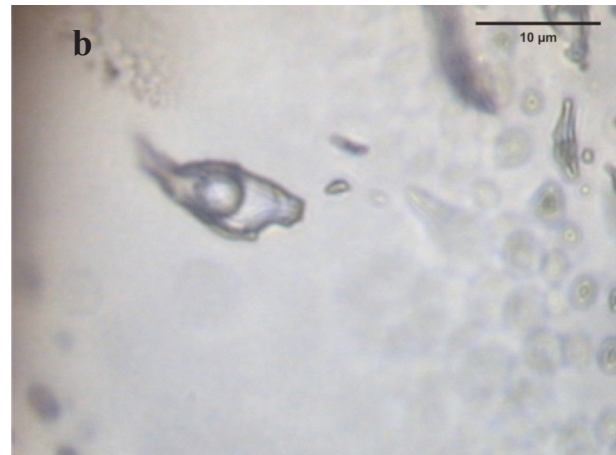
Fig 6.1b: An example of a 2 phase inclusion with a vapour bubble and a liquid in marble (Bay 22)
