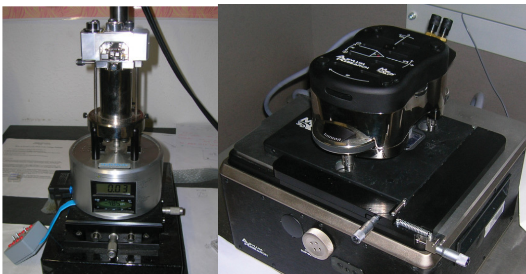
Figure 21: AFMs used in this work: Left: Digital Instruments Nanoscope IIIa Right: Asylum Research MFP 3D
