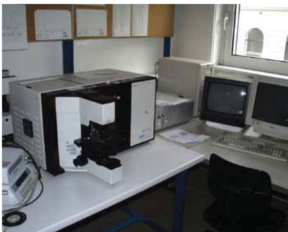
Fig. 3.4 The Raman spectrometer used for the measurements in this thesis [76].
