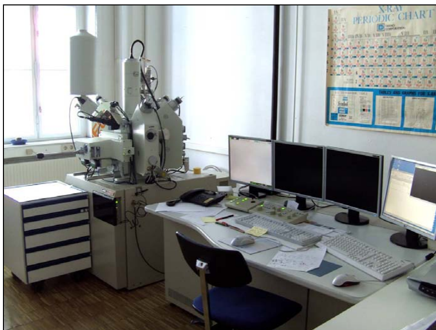
Fig. 18. Eugen F. Stumpfl laboratory (University of Leoben), electron microprobe analyses were made with a Jeol 8200 instrument (in the left part of the picture).
