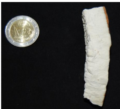
Figure 1: cm-thick carbonate scalings (left). scalings of Mg-calcite, Aragonite and Vaterite at the experiments (right)
