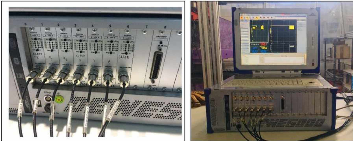
Figure 2-3: Data acquisition channel (left) and Dewesoft Computer (right).
