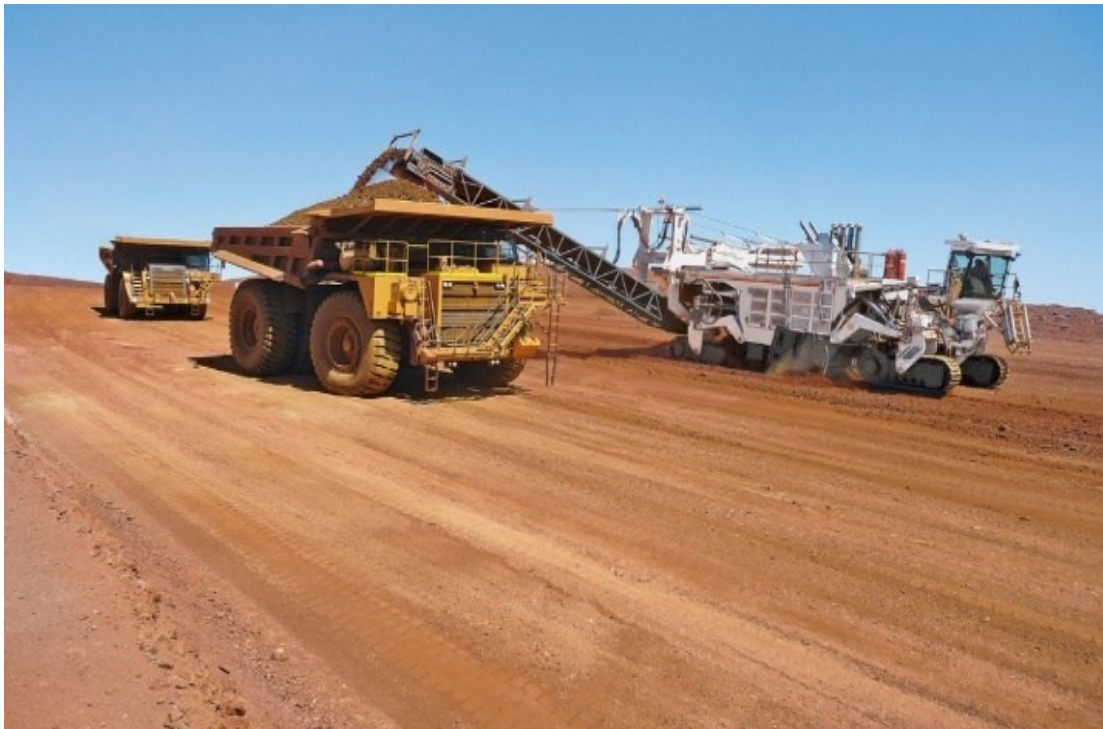
Figure 3.1-6 Direct Loading of Surface Miner [38]
