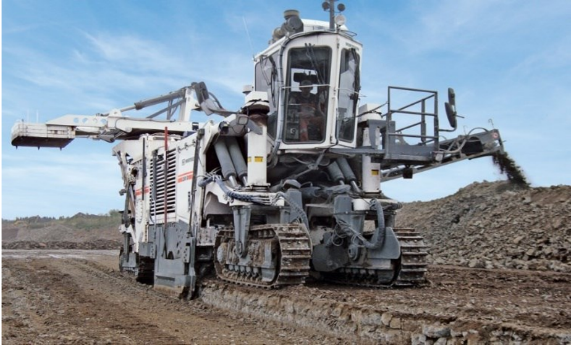
Figure 3.1-7 Windrowing of Surface Miner [39]
