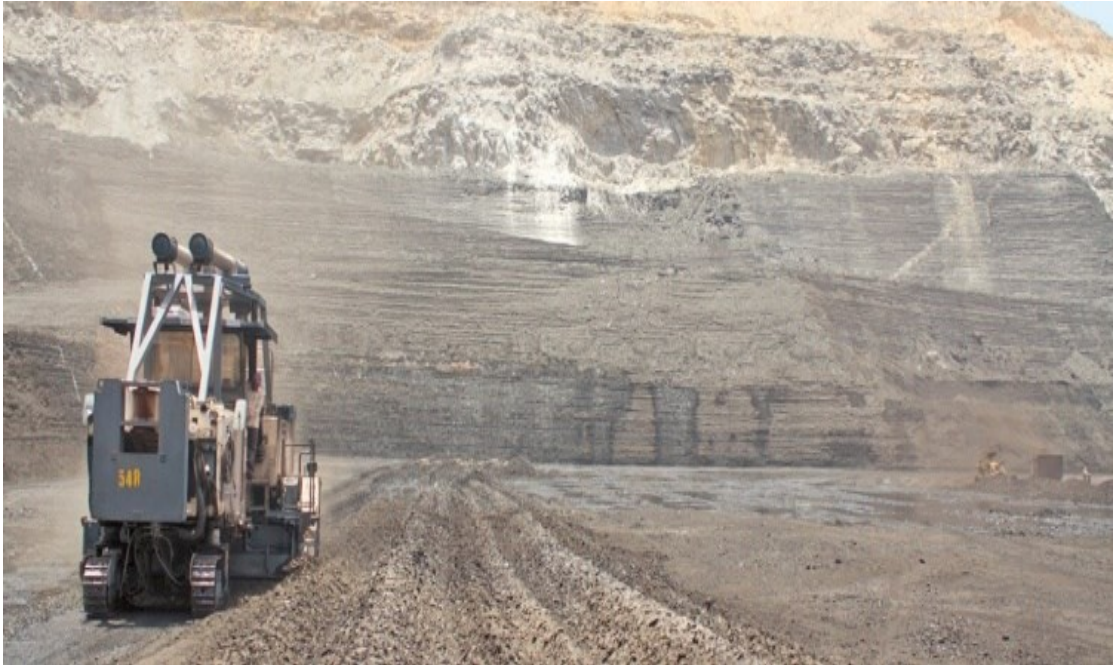
Figure 3.1-8 Side casting of Surface Miner [40]
