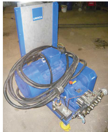
Figure 29: Left: High pressure pump with hydraulic drive [8] ; Right: High pressure pump with electric drive.
