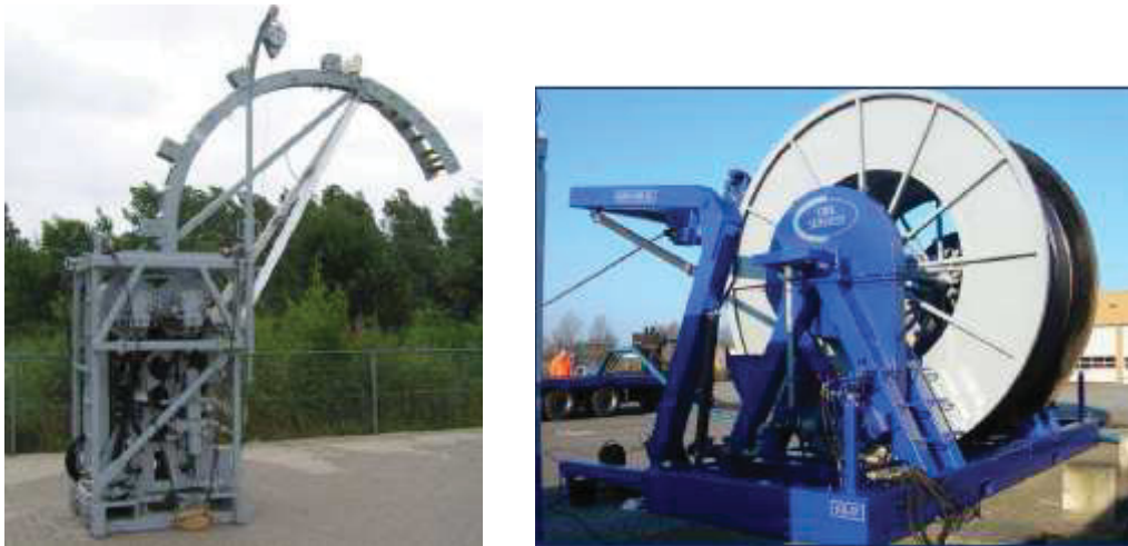
Figure 33: Left: Coil Tubing injector head with gooseneck [26] ; Right: Coil Tubing reel [26]
