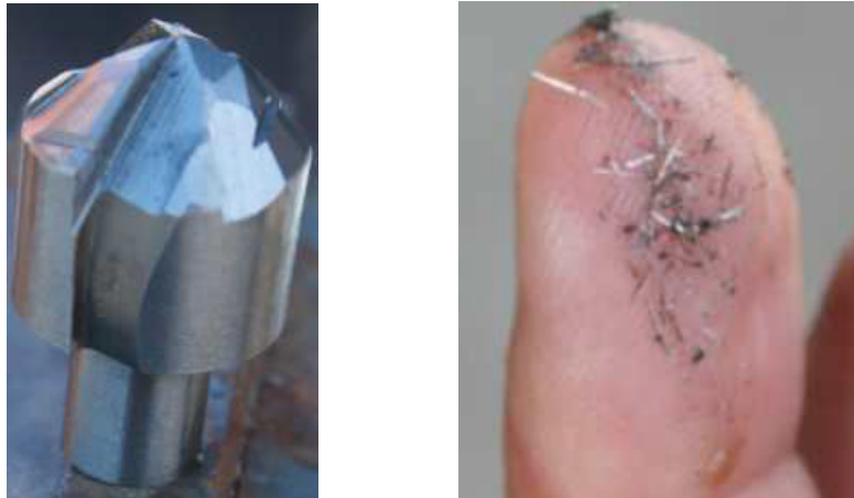
Figure 37: Left: Milling bit with three cutting edges and round tool holder; Right: Chippings.
