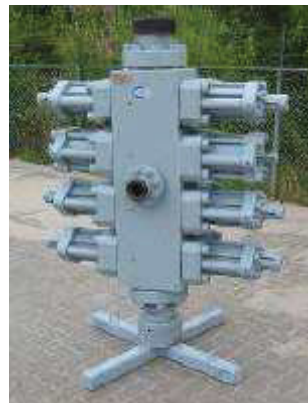
Figure 32: 4 1/16" 10.000 psi VAN OIL Blow out preventer [26]
