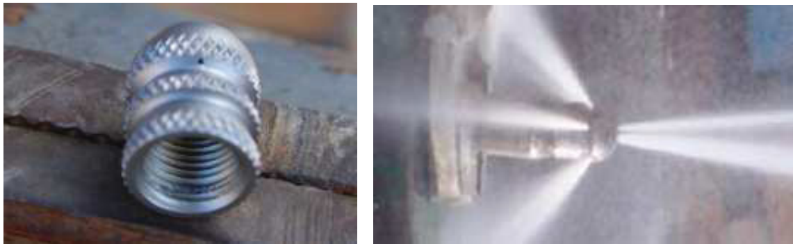
Figure 23: Left: Button Nose Nozzle for Hydro Drilling [8] ; Right: Nozzle in action [8]
