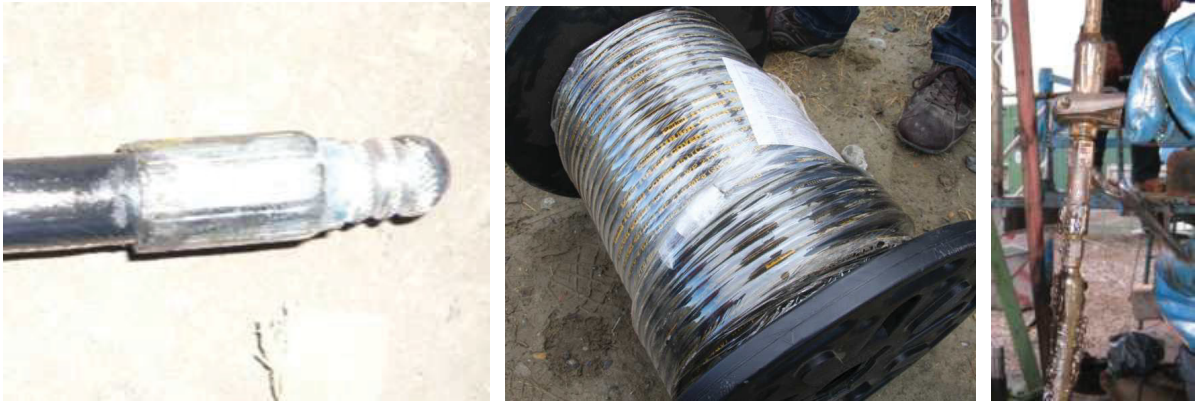
Figure 44: Left: Jetting hose connected with nozzle; Between: Jetting hose; Right: Jetting hose connected with Coil Tubing.
