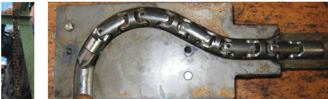
Figure 38: Left: Cardan shaft in pendulous state; Right: Cardan shaft inside the deflector shoe.
