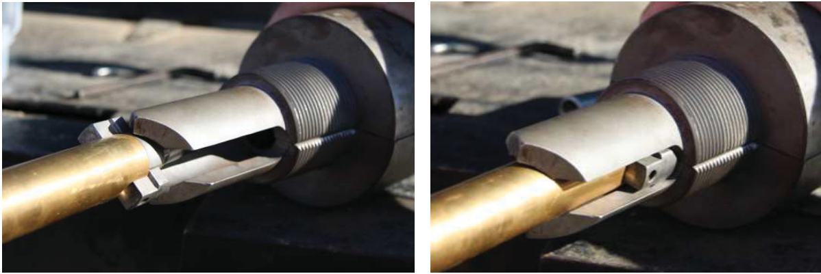
Figure 35: Left: Torque supply moves in the deflector shoe; Right: Torque supply is fixed in the deflector shoe.
