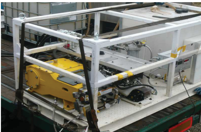
Figure 29: Left: High pressure pump with hydraulic drive [8] ; Right: High pressure pump with electric drive.
