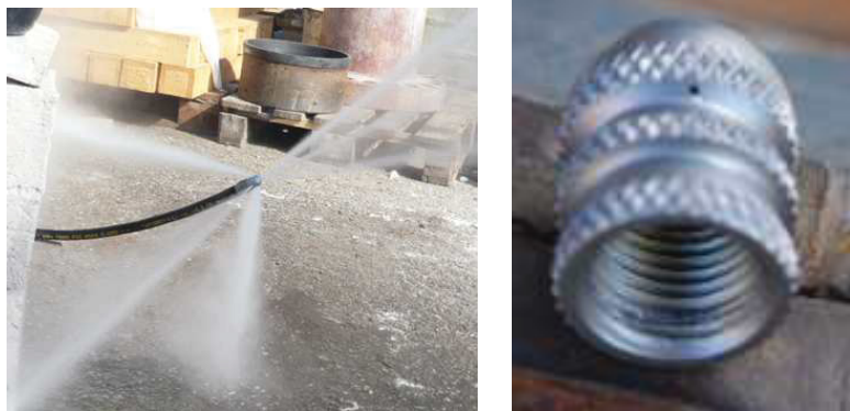
Figure 43: Left: Button Nose nozzle in action; Right: 1/8" Button Nose nozzle for Hydro drilling.
