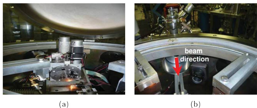
Fig. 14: (a) Sample holder adjusted in the chamber for the room temperature experiment. (b) The arrow mark the direction of the beam within the chamber.
