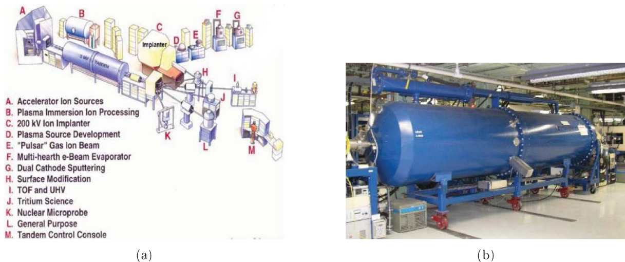
Fig. 12: (a) Ion Beam Material Laboratory with a tandem ion accelerator, an ion implanter and several beam lines attached [24]. (b) Image of the tandem ion accelerator at the IBML [24].
