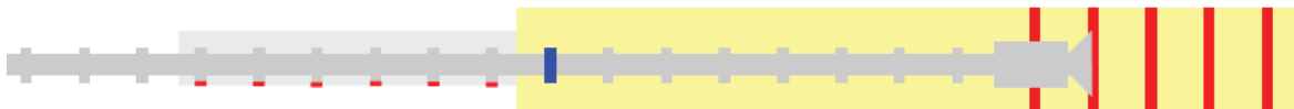
Fig. 100 Position of the tool joint during encounter of the second stringer: on-spot wear is created at the same relative positions
