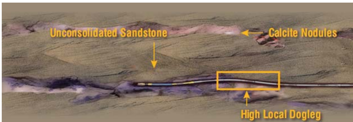
Fig. 35 Locally high dogleg due to hard calcite stringers / nodules [3]
