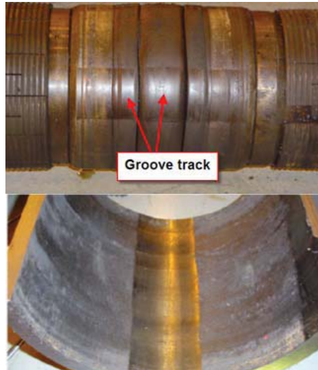
Fig. 71 Retrieved swell packer set in severely worn casing
