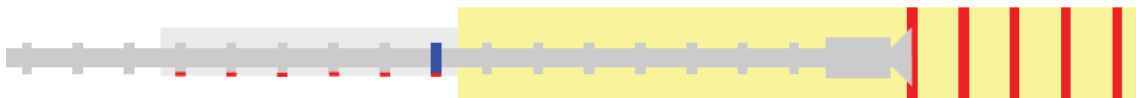
Fig. 99 Position of the tool joint during encounter of first stringer: on-spot wear is created for the first time
