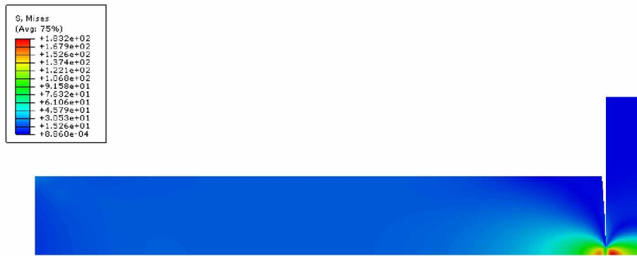
Fig. 6.40: Mises equivalent stress distribution at a normal load of 1500 N
