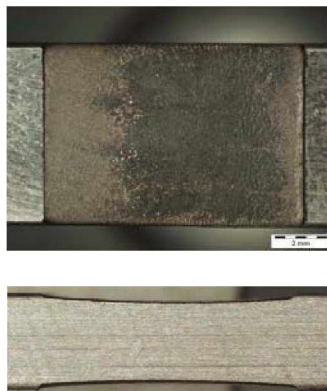
Fig. 6.52: Fretted surface of a specimen at a stress level of 200 MPa
