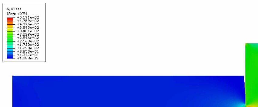
Fig. 6.41: Mises equivalent stress distribution at a normal load of 1500 N and stress amplitude of 300 MPa
