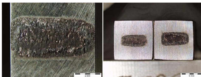
Fig. 6.17: Fretting wear damaged surface of a recrystallization-annealed microstructure
