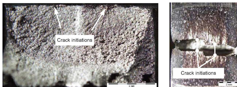
Fig. 6.23: Fracture and fretting damaged surface of a solution treated specimen at 300 MPa
