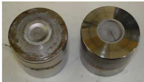
Figure 3.8.: Anvil surface after deforming some samples at 200°C (left) compared with a recently machined anvil only used for RT deformation (right).
