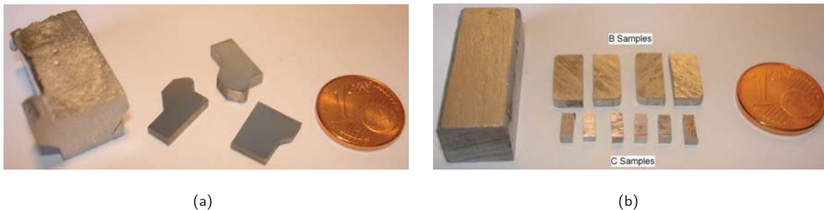
Figure 2.4.: Samples of raw material from, excess material of the sprue for A samples(a), homogenized material for B and C samples(b).
