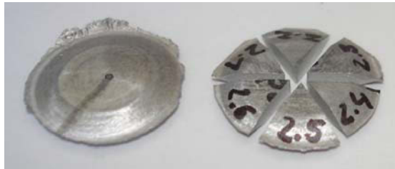
Figure 3.9.: HPT deformed samples: as deformed (left) and one sectioned to be aged (right).
