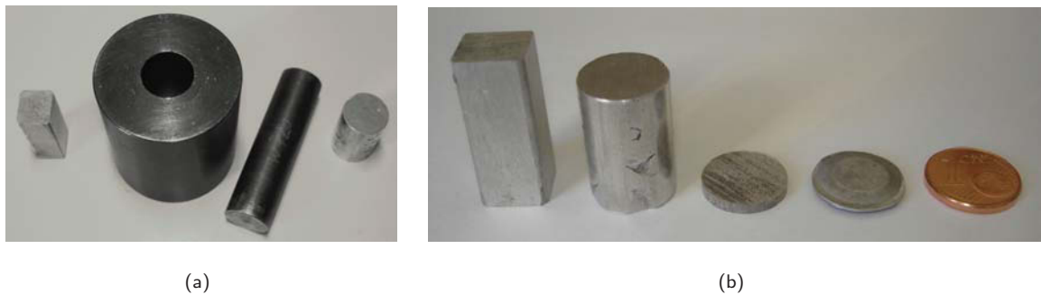
Figure 3.6.: (a) Tool for compression of bars to cylinders. (b) Production steps of samples for HPT experiments. From left to right: cuboid of homogenized material \rightarrow compressed to a cylinder \rightarrow cut into slices \rightarrow pre-shaped with HPT dies; 1 €-cent \varnothing 16.25 mm.
