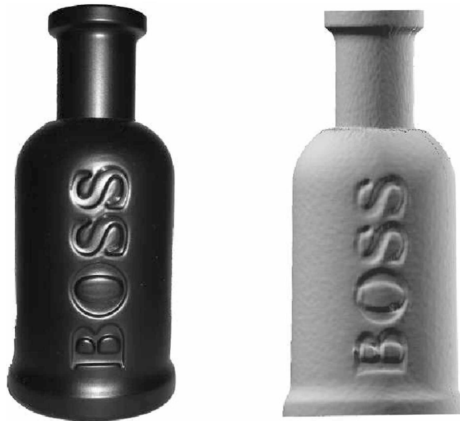
Figure 3.3: The above object has an axis of rotation around which it is predominantly invariant. Left: photograph of the object. Right: result of the scan with the proposed system.
