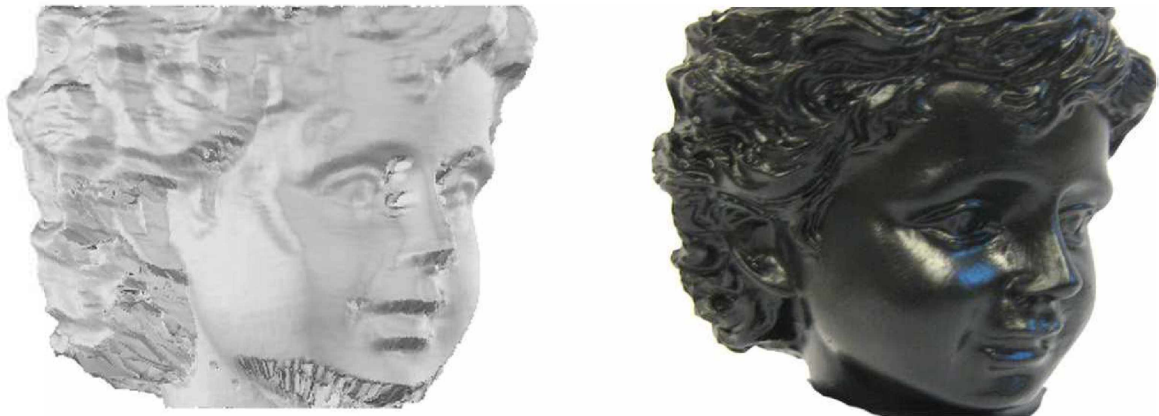
Figure 6.11: Scanned head of a little statue (left: photograph, right: reconstruction).
