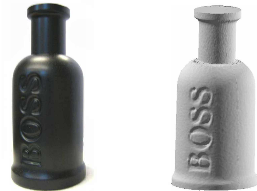
Figure 6.8: Example of the scan of a parfum bottle (left: photograph, right: reconstruction).
