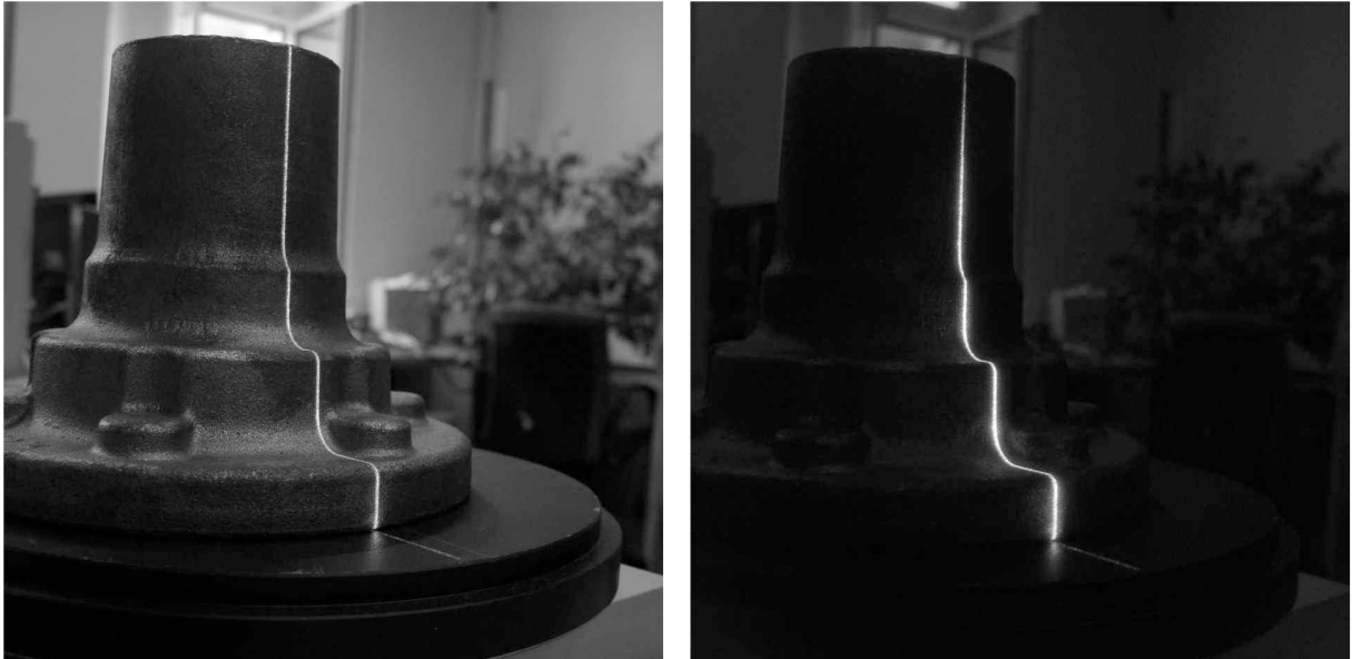
Figure 6.14: Image taken without an optical interference filter (left) and image taken with filter (right).
