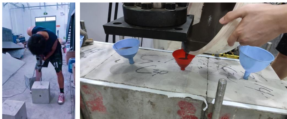
Figure 12 Full-length grouting process
