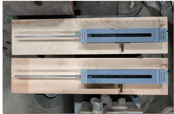
(b) Displacement meter
