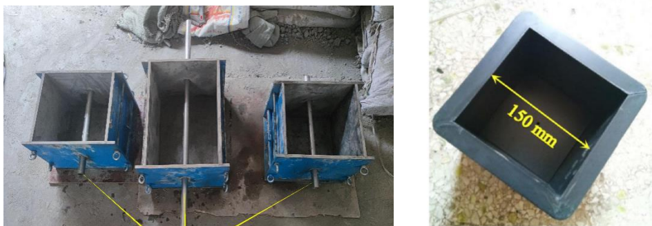
Figure 6 Concrete casting moulds
