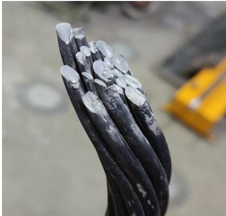
(a) Shear breakage of cables
