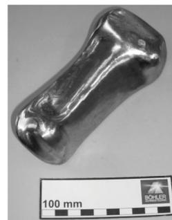
Fig. 4. Pre-form of a turbine blade manufactured by upsetting both sides of a cylindrical bar and subsequent side pressing to the final shape.<sup>[17,27,28]</sup> After forging the surface of the pre-form was ground.
