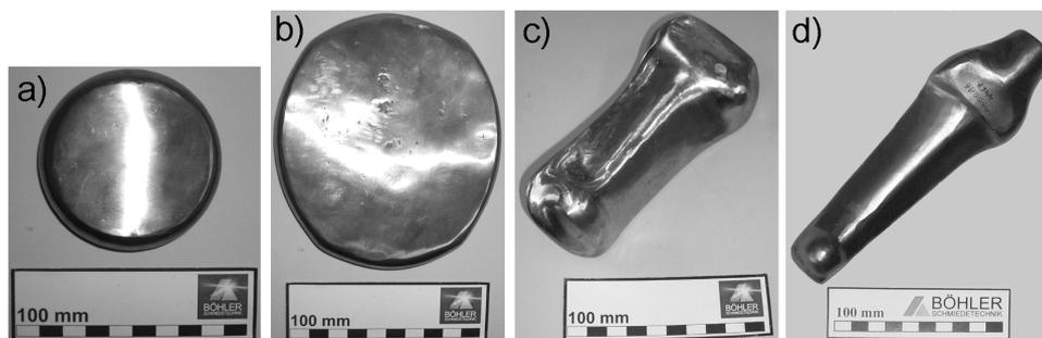
**Figure 3.** TNM™ billets after (a) upsetting to an overall strain of 0.7 and (b) after side pressing to an overall strain of 1.3. Photographs (c) and (d) show different TNM™ blade pre-forms manufactured by upsetting both sides of a cylindrical bar and subsequent side pressing to final shape (3-step forging process). After forging the surface of the depicted examples was ground.
