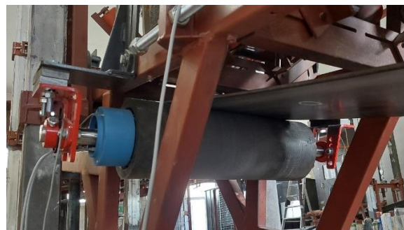
Figure 3 PrimeTracker pressed onto the carrying side
