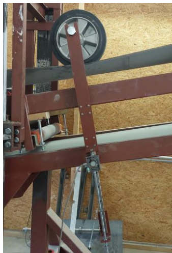
Measuring the contact force of the wheel onto the belt
