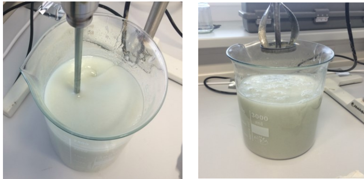
Figure 11: BEER® fracturing fluid without glass beads (on the left) and with glass beads (on the right)
