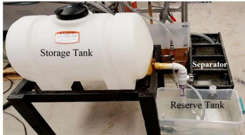
Figure 2.3 - Mud circulation and filtration system (Bilgesu et al., 2017)
