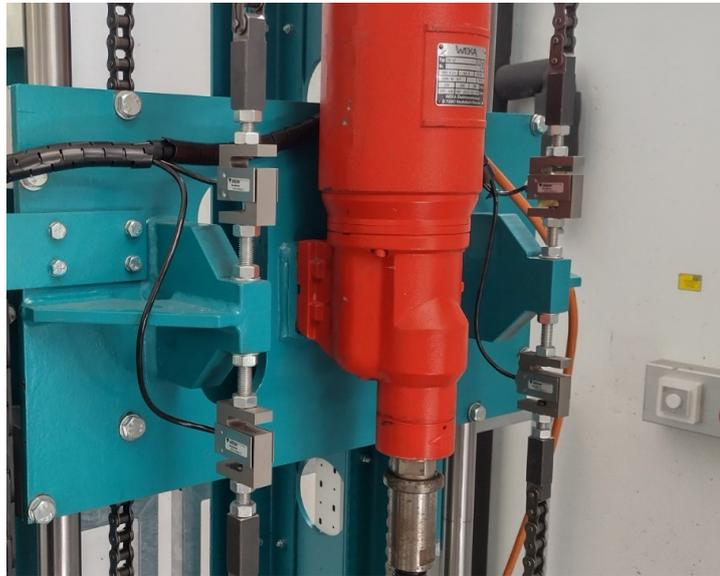
*Figure 3.9 - Four S-type load cells*
