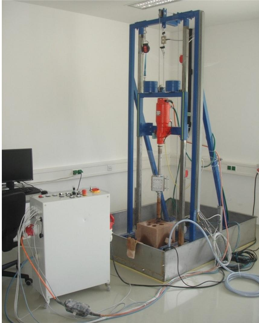
*Figure 3.1 - Initial setup of MiniRig (Esmaeili et al., 2012)*
