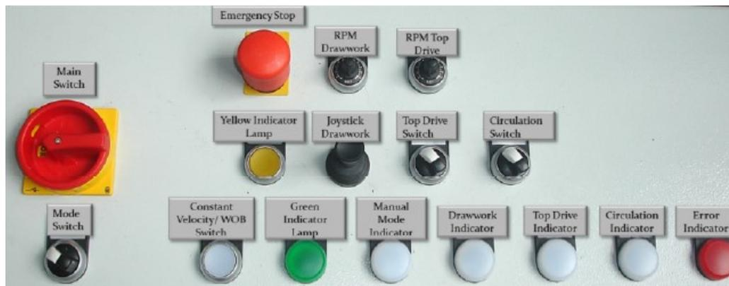
Figure 3.4 - MiniRig driller's console(Esmaeili, 2013)
