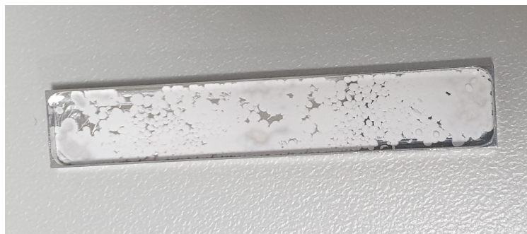
Figure 40: PTFE sample with too low sample volume after completing the DMA.
