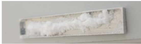
Figure 30: Heaped TPE powder in the Powder Pocket.
