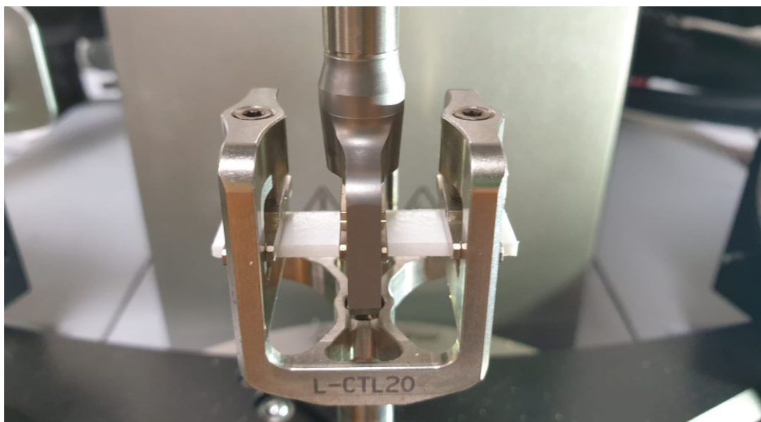
Figure 20: PVC-sample fixated in the CTL-20.
