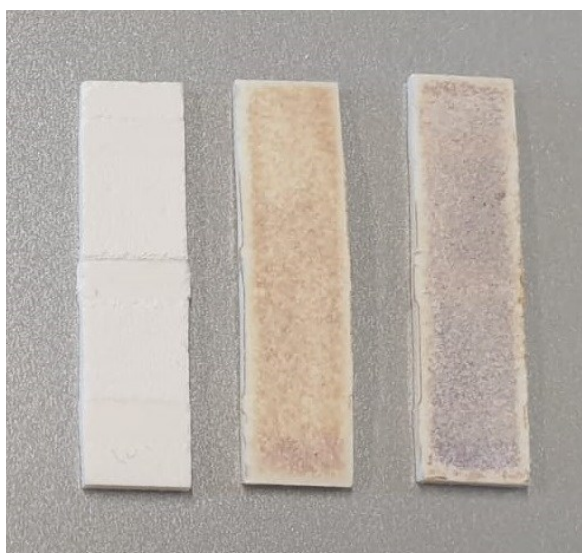
Figure 18: Discoloration due to decomposition of the PVC samples produced at different temperatures: 265 °C for 3,5 min (right), 220 °C for 5 min (center) and no obvious decomposition at 180 °C for 7 min (left).
