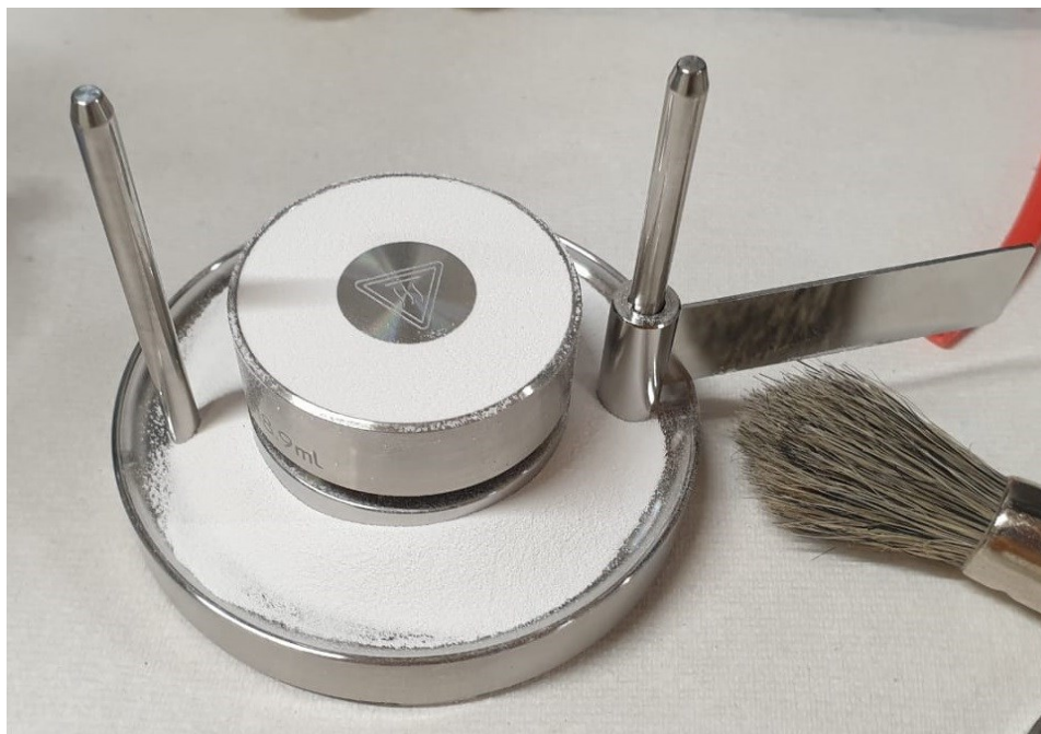
Figure 21: Preparation tool for the volumetric filling of the shear cell.
