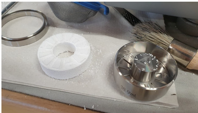
Figure 53: PTFE Powder keeping its shape after testing at 30 °C due to strong interaction forces caused by fibrillation.
