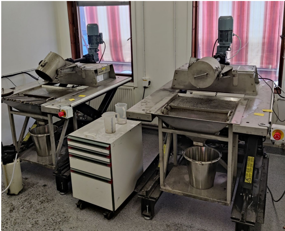
Figure 6. Laboratory tumbling mills used for the comminution tests at LKAB's mineral processing laboratory in Kiruna
