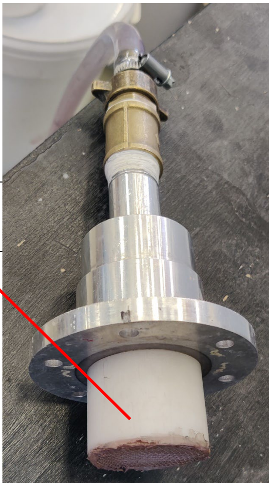
Figure 26. Lower part of the aluminium container with distance holder
