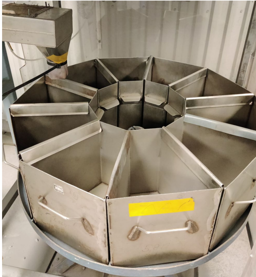
Figure 5. Rotating splitter at LKAB's laboratory for physical testing in Kiruna
