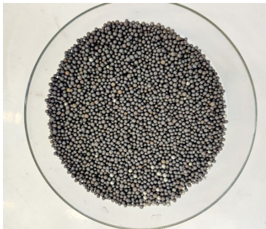
Figure 25. Steel balls used as the Matrix.
