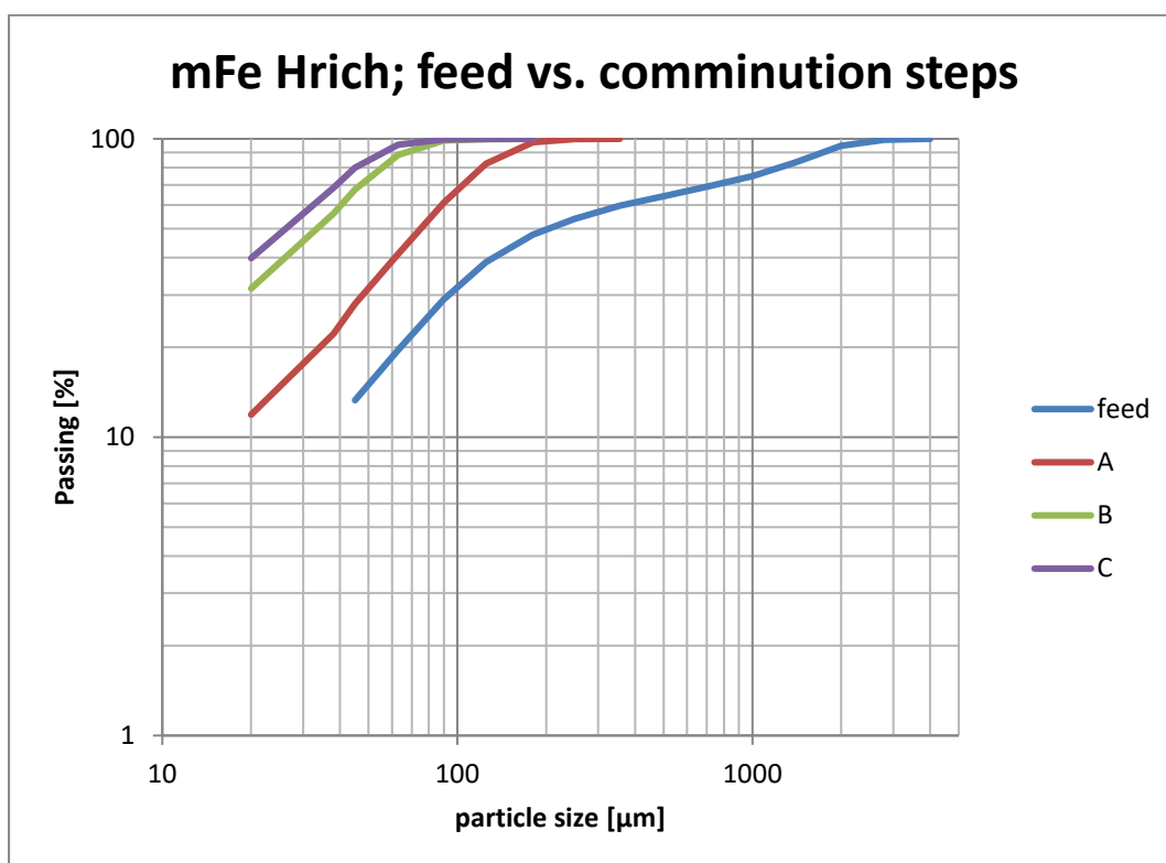
Figure 69. MFe Hrich: Particle size distribution of the feed and the grinding products after comminution steps A, B and C.
