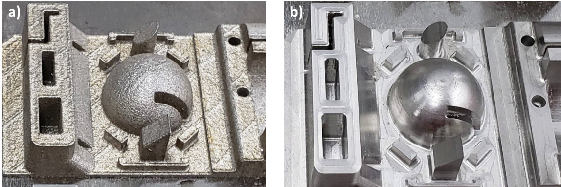
Figure 13: Additively manufactured mold a) before and b) after postprocessing (CNC milling) [41].
