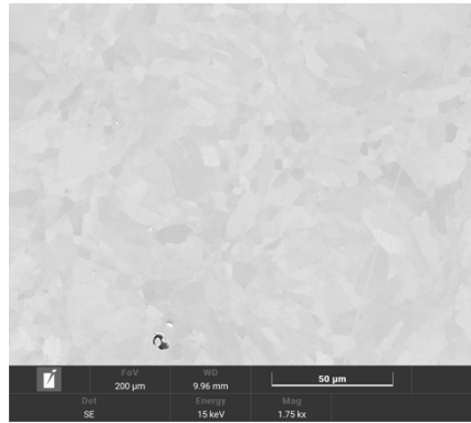
Transversal cut of sample N: 200 W and 800 mm/s
