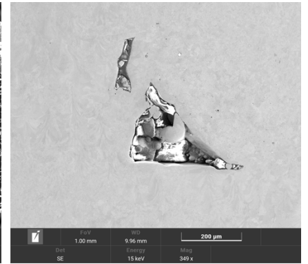
Longitudinal cut of sample N: 200 W and 800 mm/s
