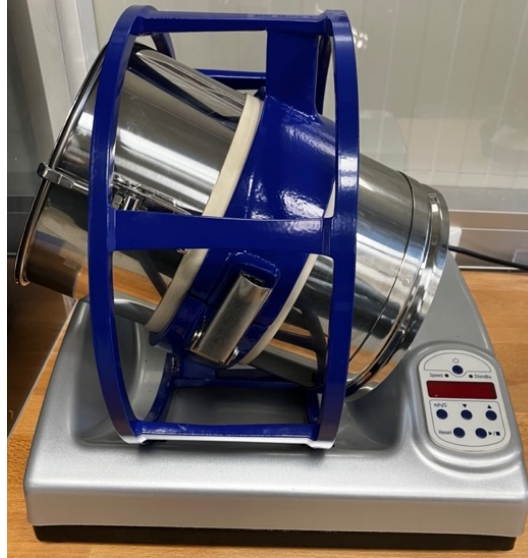
Figure 15: Drum hoop mixer JEL RRM Mini-II by J. Engelsmann AG used for powder mixing.
