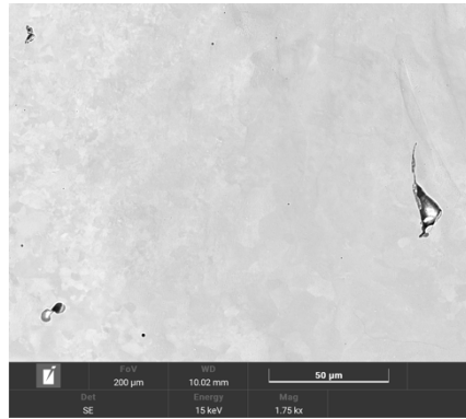
Transversal cut of sample P: 200 W and 1000 mm/s
