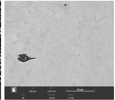
Longitudinal cut of sample P: 200 W and 1000 mm/s
