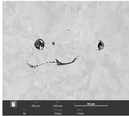
Transversal cut of sample O: 200 W and 900 mm/s
