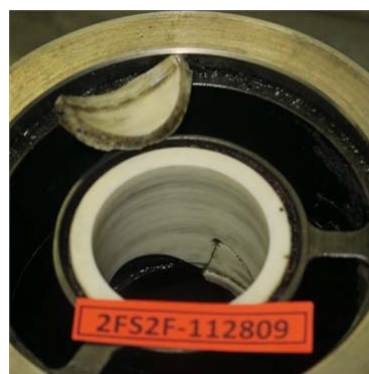
Figure 36 - Broken Zirconium bearing
