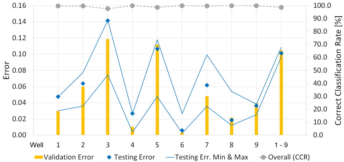
Figure 53 - Model evaluation of artificial data set based classifiers for pump wear: Task 1, Training arrangement “single” & “all together”
