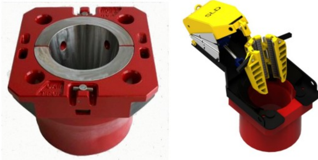
Figure 39: The bushing comes with 3 different insert bowls, one capable of handling 2 3/8 in to 8 5/8 in OD tubulars. The master bushing can be equipped with pneumatic slips at the corner bores or a bit breaker adapter plate ([41],[42]).
