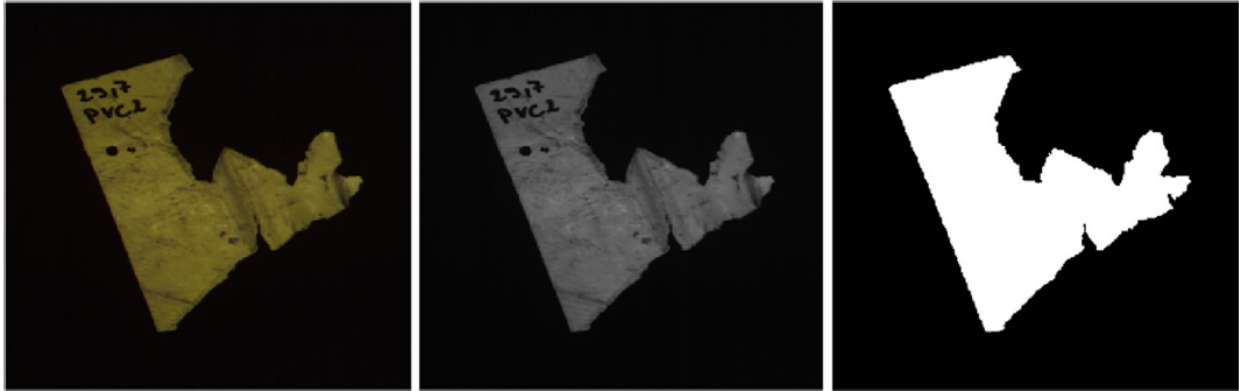
Figure 2: RGB image (left), greyscale image (middle), and binary image (right) of singlified waste particle.
