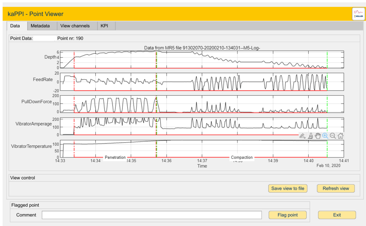
Figure 6: Visualization of a selected sub set of the real time machine data; here for point 190. The real time machine data for each point in Fig. 4 and Fig. 5 are available in the system. They are directly linked to support the visualization of detailed machine behavior. The data is automatically segmented to indicate the penetration and compaction phases. This example shows a pre-drilled point, identified by the fact that the vibrator enters the ground without significant pull down force while the electric motor was even turned off. Anomalous points can be flagged and commented in this view.
