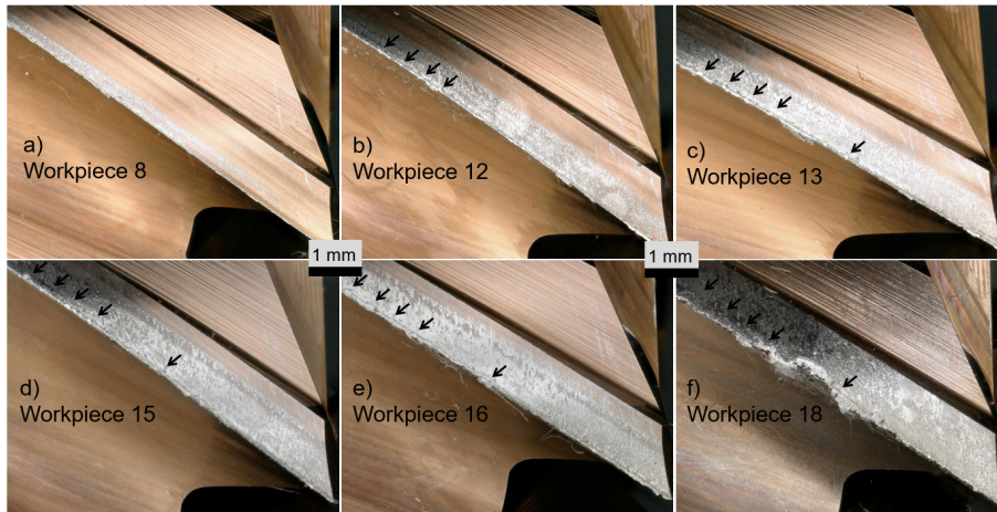
Figure 18: Digital images of the milling tool after having milled different amounts of workpieces. Black arrows indicate the positions of breakouts at the cutting edge that influence the distributions of the sensor signals discussed in the current work. The increase in wear and damage feature size is visibly increasing with the number of workpieces milled, which is expected.
