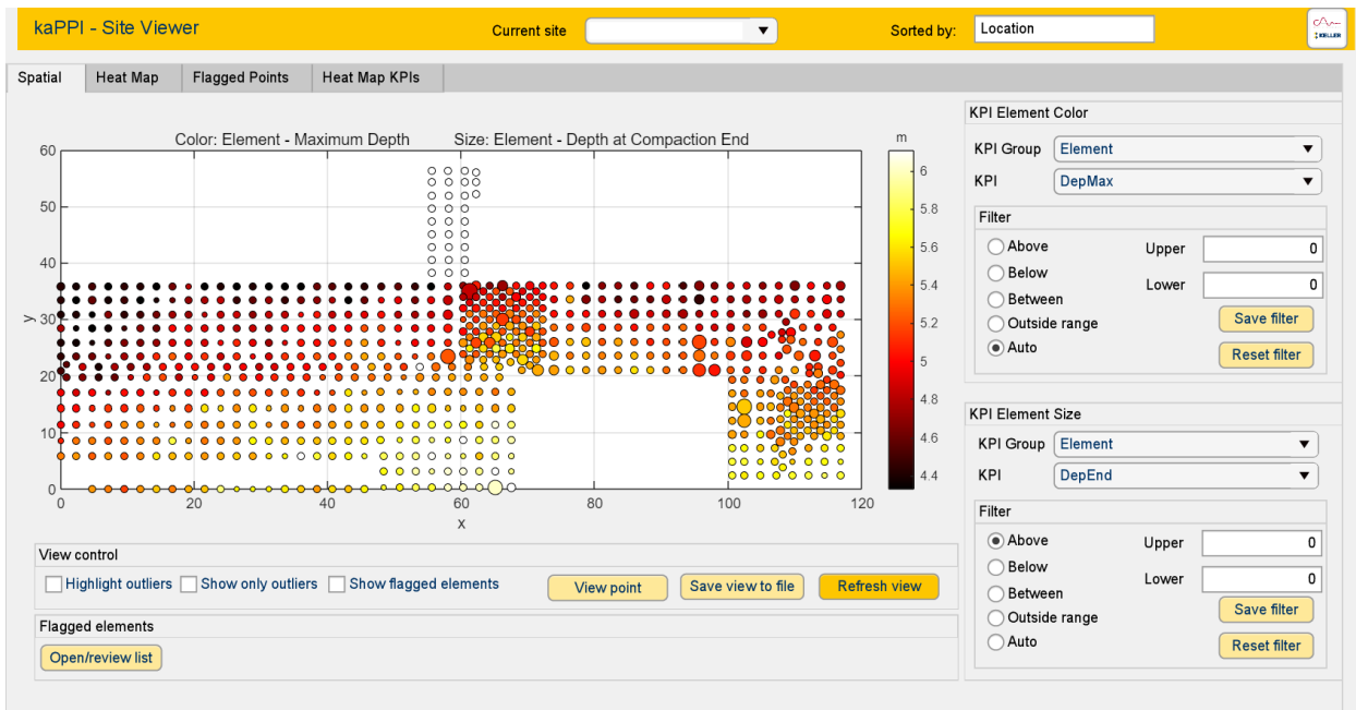
Figure 4: Geo referenced simultaneous presentation of two KPIs - one as color, one as symbol size for each point (column) of a construction site. Note: in this example, a series of planned but not executed points can be seen at the top (white circles). Furthermore, a systematic variation of the KPI (color) can be seen from the top left towards the bottom right; this reveals a systematic change in underground properties. The panels on the right permit the definition of filters for the KPIs, with the aim of detecting and marking outlier points. Additionally, points manually flagged as being exceptional can be indicated.
