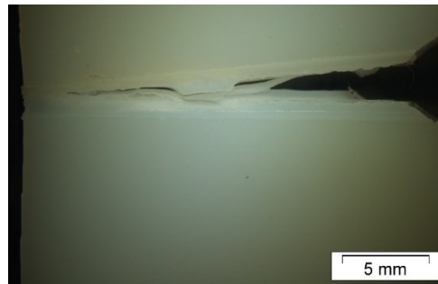
Figure 32: Front side of a HIPS B CT specimen with side grooves tested in oil.
