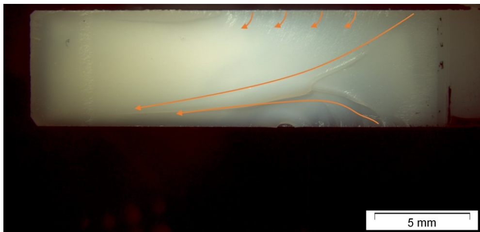
Figure 42: Different crack tips in HIPS B when tested in oil.
