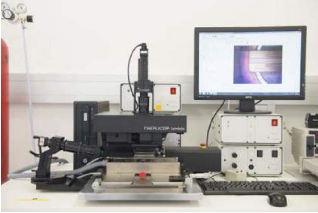
Figure 3.4. Fineplacer setup to prepare die bonded samples.
