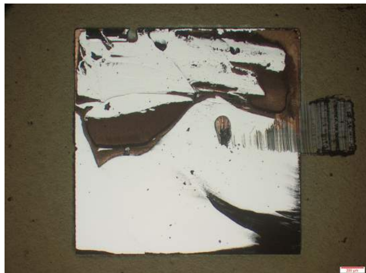
Figure 5.8. Optical microscope image of sample 3 of CP3 after SAM imaging and the shear test.
