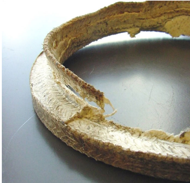
Figure 4.47: Extrusion of a packing ring [24]
