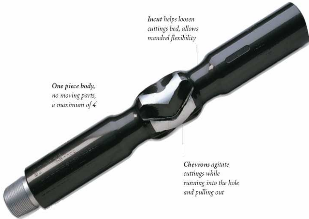
Figure 49: Representation of the Cuttings Bed Impellers
