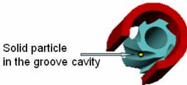
Figure 39: Lifting effect of a solid particle
