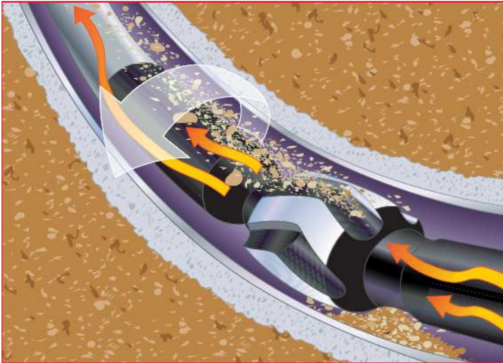
Figure 50: mechanical agitation of cuttings bed with the CBI
