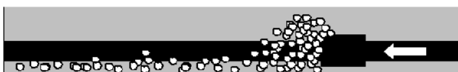
Figure 13: Pack-off while pulling the BHA out of the hole
