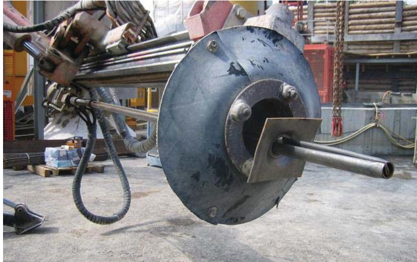
Figure 55: Hardi bolt on boom and ready for installation [46]
