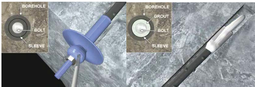
Stage 2 injecting grout into the bore
