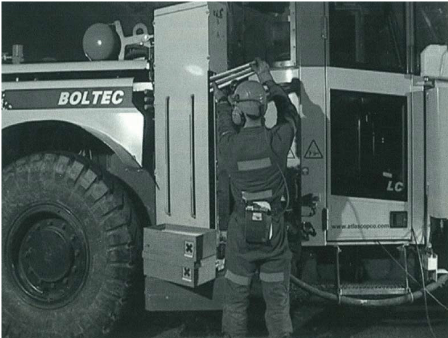
Figure 95: Filling Magazine with resin cartridges [73]
