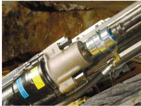
Figure 97: Integrated rotary injection adapter fixed on the boom [36]
