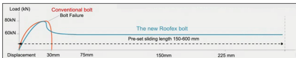
Figure 51: The displacement curves of conventional bolt and Roofex under dynamic application [44]
