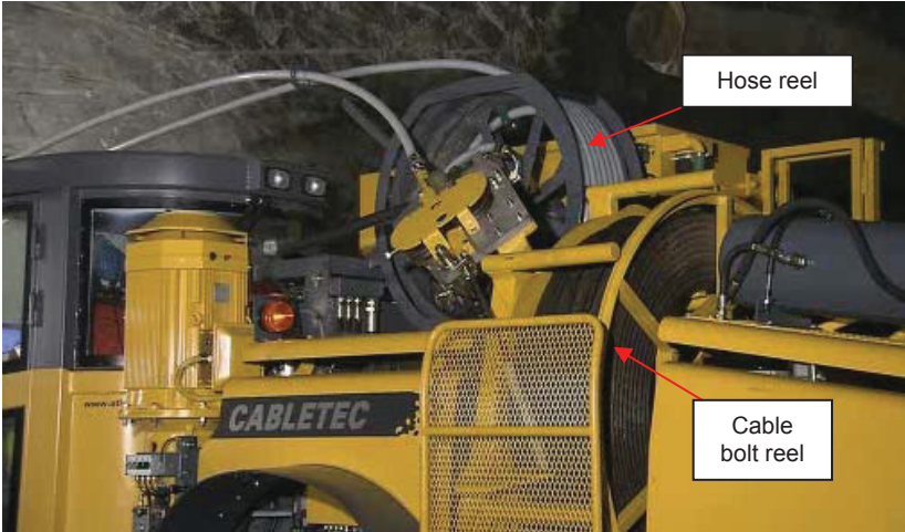
Figure 103: Cable reel and grouting hose reel [44]
