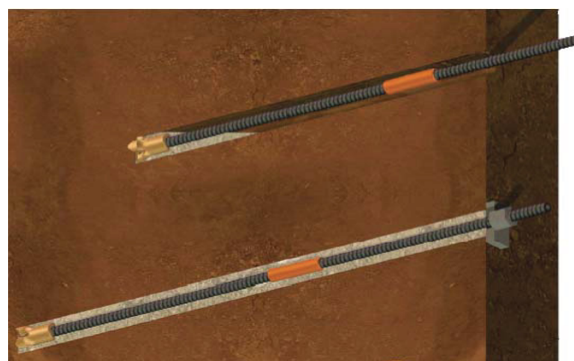
Figure 38: Self-drilling anchor during installation [37]
