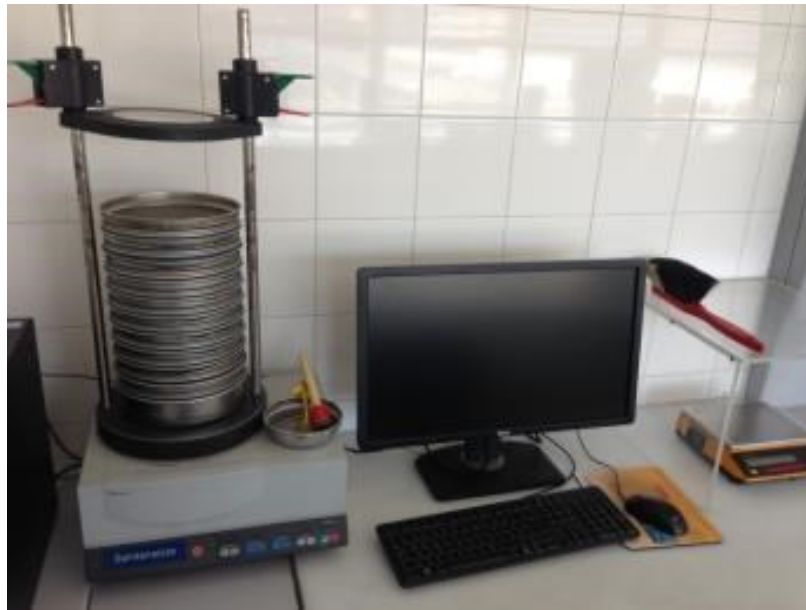
Figure 3-1: Sieve shaker used for granulometry and scale.
