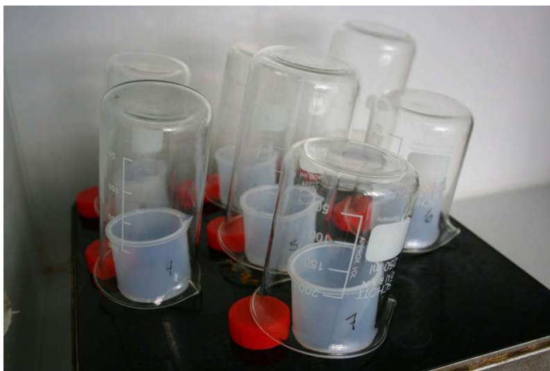
3. Eluent evaporation after cation exchange matrix separation
