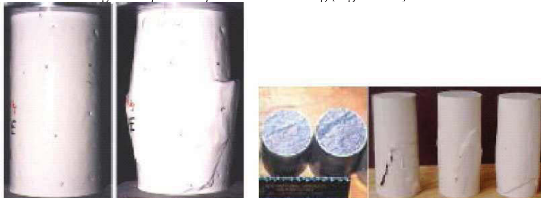
Figure 3-69 Concrete and rock samples before and after compression failure (Archibald, 2001)
