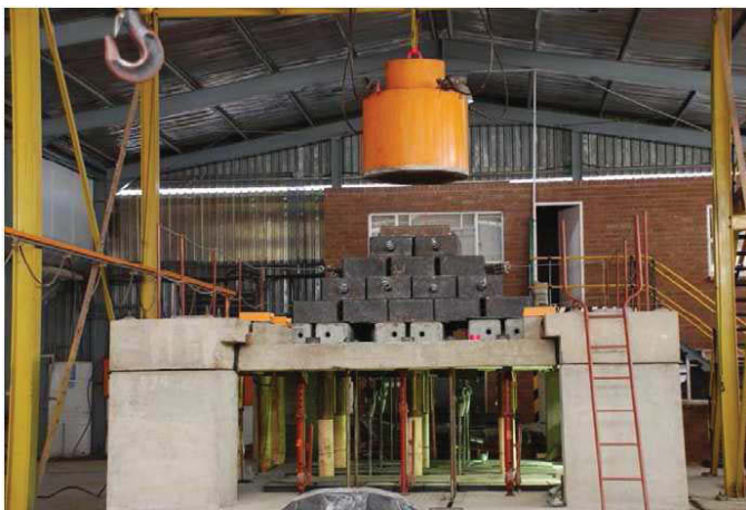
Figure 3-96 SIMRAC dynamic testing rig (Li, 2008)
