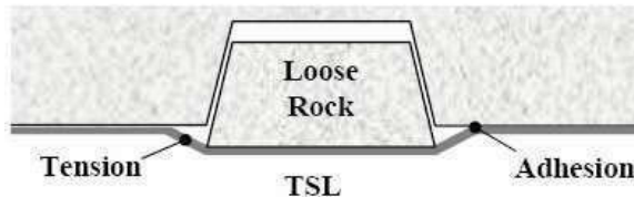
Figure 3-61 TSL supporting a loose rock (Yilmaz, Saydam and Topper, 2003)
