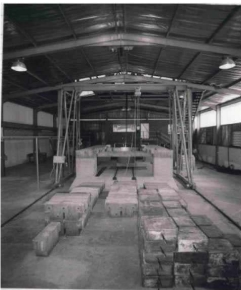
Figure 3-98 Testing rig, showing the stope with the drop weight temporarily berthed at the centre of the stope floor (Ortlepp, 2000)
