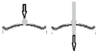
Figure 2-4 Sketch for plate testing (van Sint Jan and Palape, 2007)
