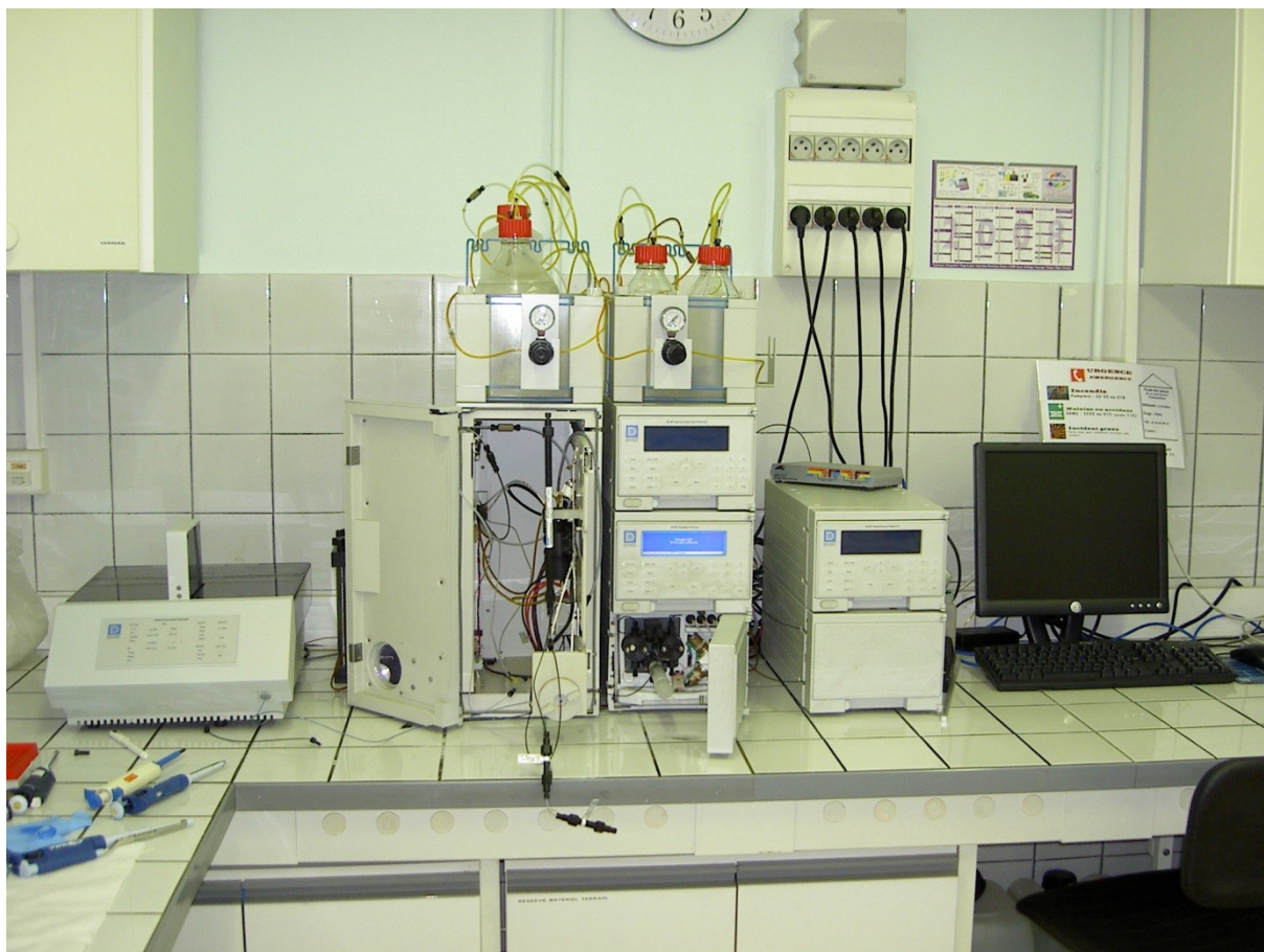
Figure 22: LC DIONEX DX 500 with the gradient pump GP40 and the electrochemical detector ED40
