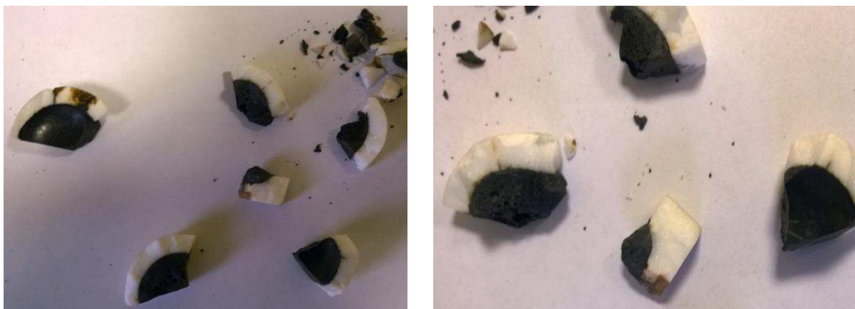
Figure 7-7: Parts of MgO crucible with industrial slag at 1500°C and 1600°C
