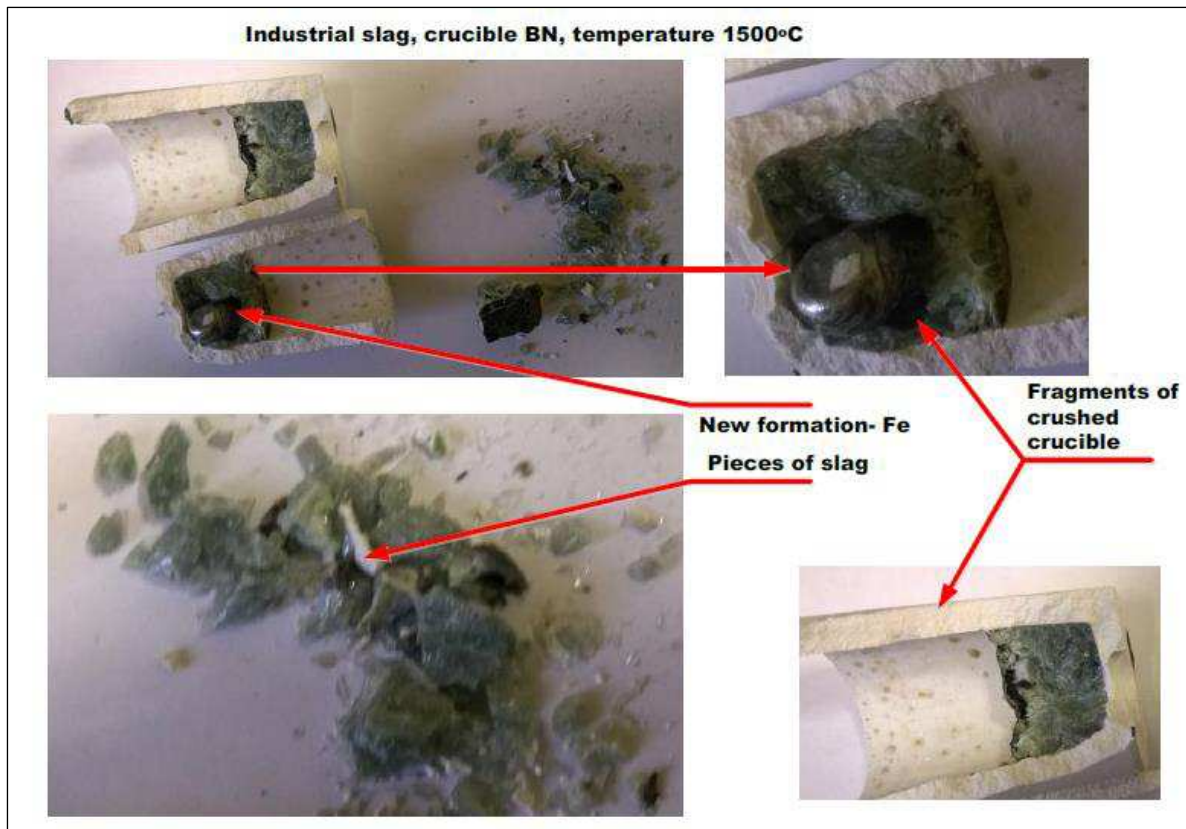
Figure 7-2: Pictures of broken BN crucible after test with LD slag at 1500°C
