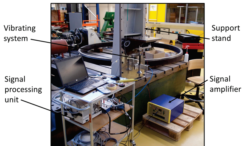
Figure 5.1: Picture of the built up test stand
