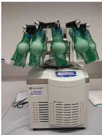
Figure 25: Fully laden ALPHA 1-2 LD plus freeze dryer
