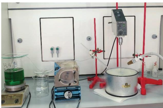
Figure 23: Freeze drying setup – shock-freezing in liquid nitrogen
