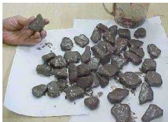
Figure 2.2: Sloughing rock chunks, frequently associated with more ductile rocks, rounded by tumbling /7/
