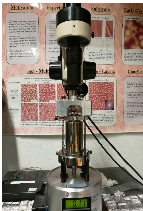
Figure 9: Photography of the Multimode AFM used in this thesis
