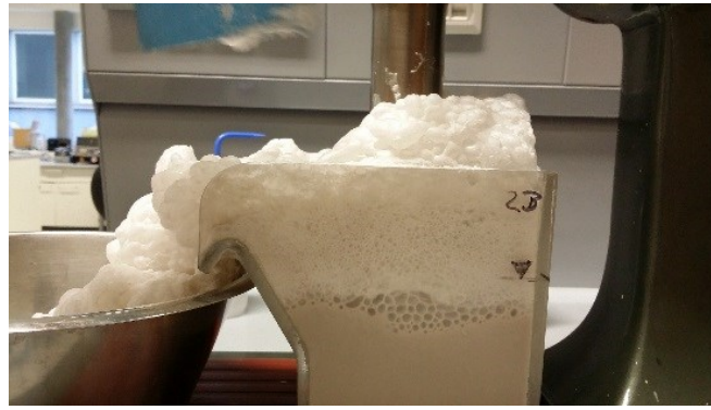
Fig. 5-5: Conventional flotation test on talc
