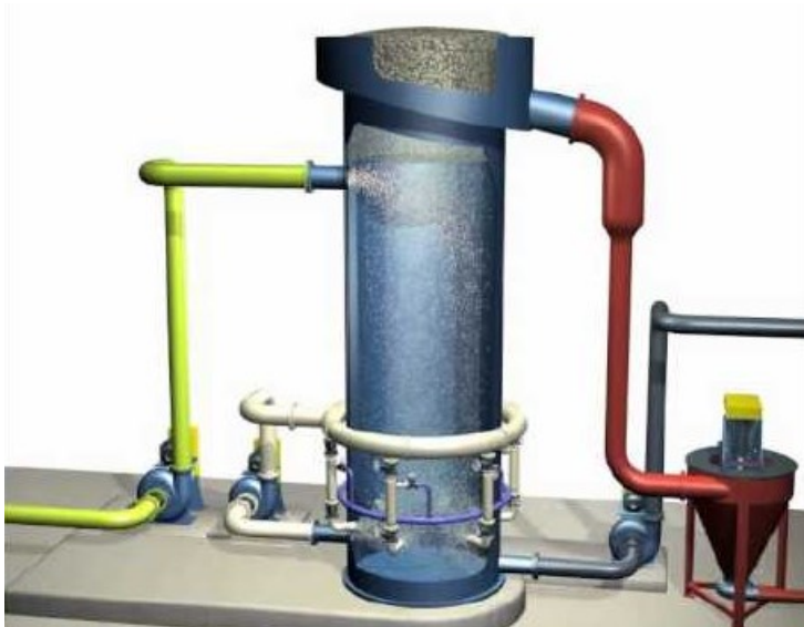
Fig. 1-5: Industrial Metso Flotation Column [5]
