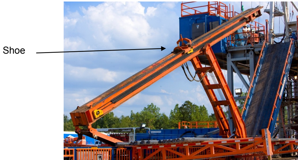
Fig. 16.3 Sample picture of a hydraulically operated catwalk, ([23])
