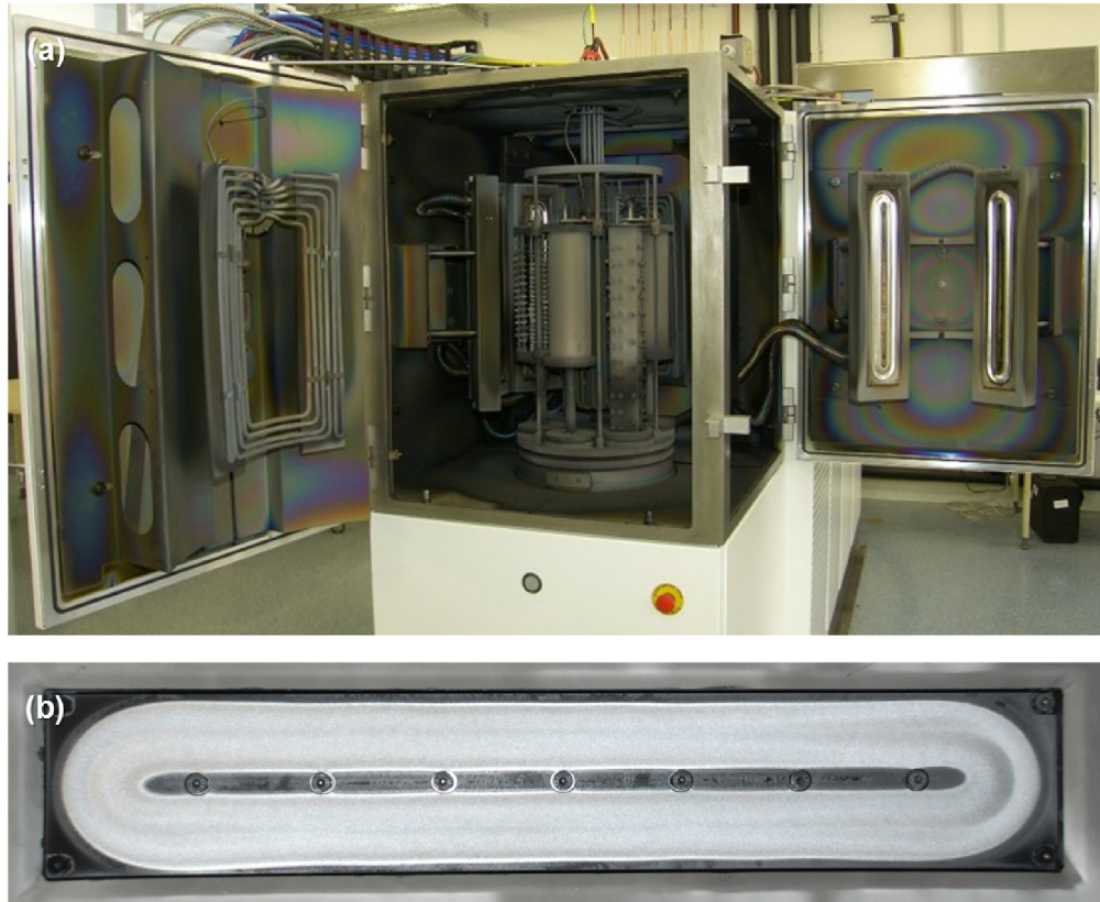
Figure 1.2: Picture of (a) the industrial-scale magnetron sputtering CemeCon CC800/9MLT deposition plant used and (b) a powder metallurgically processed \text{Cr}_{0.45}\text{Al}_{0.45}\text{Si}_{0.10} target. The carousel where the substrates were mounted is located in the center of the chamber.
