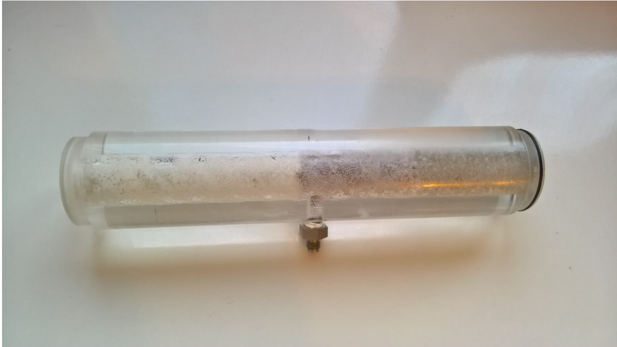
Figure 62: Flow Tube with insoluble Content after Consolidation
