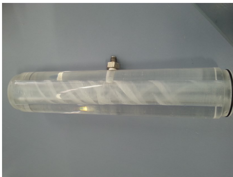
Figure 33: Flow Tube with Sidewall Adaption and O-Ring
