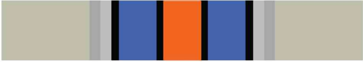
Figure 21: Cross-section formation — wellbore. From left to right: formation (brown, dotted), cement (gray — dotted part represents cement penetrated into formation), casing (black), cold water stream downwards (blue), tubing (black) and warm water stream upwards (orange).
