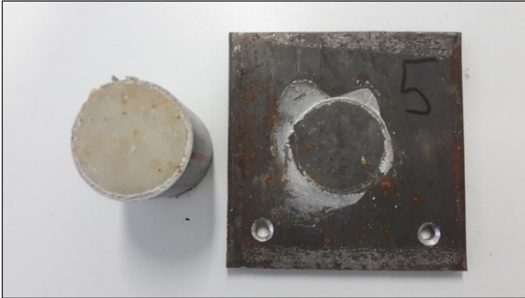
Figure 30: Test sample 5 Steel/Cement
