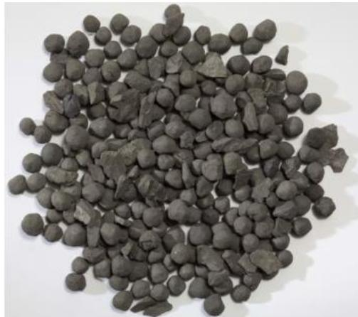
Abbildung 4: Direct Reduced Iron Pellets [5]
