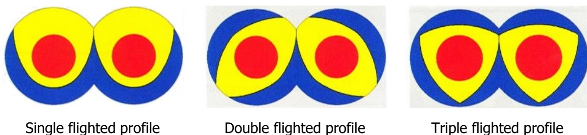
Figure 3.2: Number of flow channels and free volume in single and multiple-flighted screw elements (Kohlgrueber, 2008)
