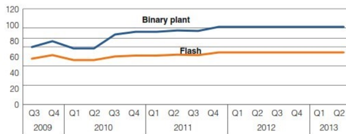
Fig. 2.18: LCOE development of geothermal electricity production in Flash- and Binary Cycle Power Plants (WEC, 2013).
