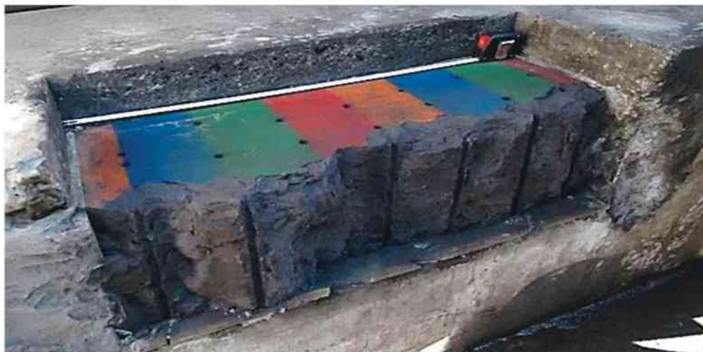
Figure 61: Front view after blasting of 2nd burden deviation pattern CH03B02, row 1
