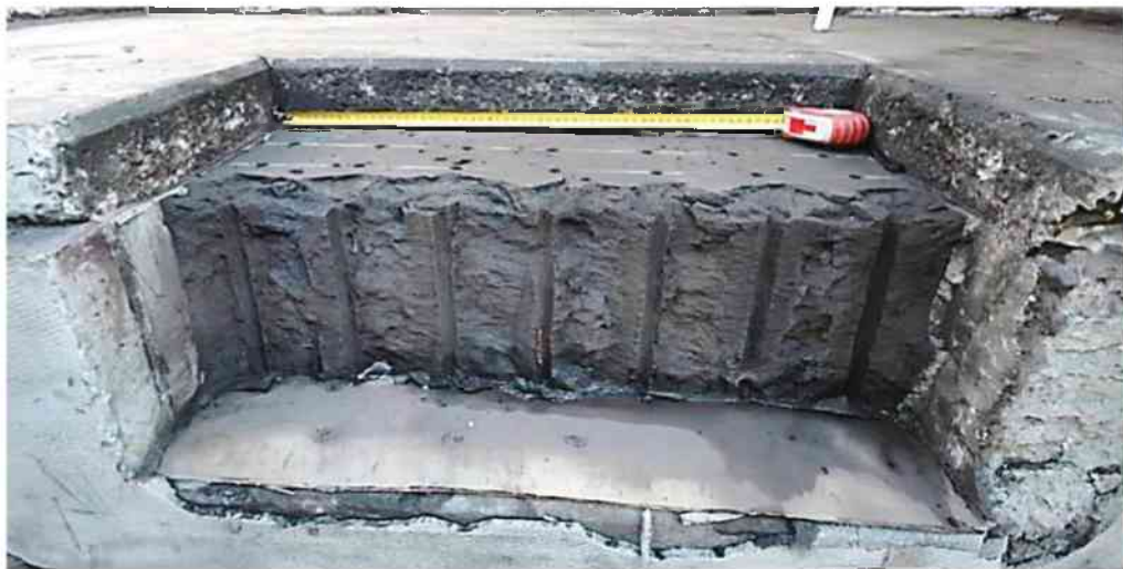
Figure 59: Front view after blasting of Reference block B06 row 1
