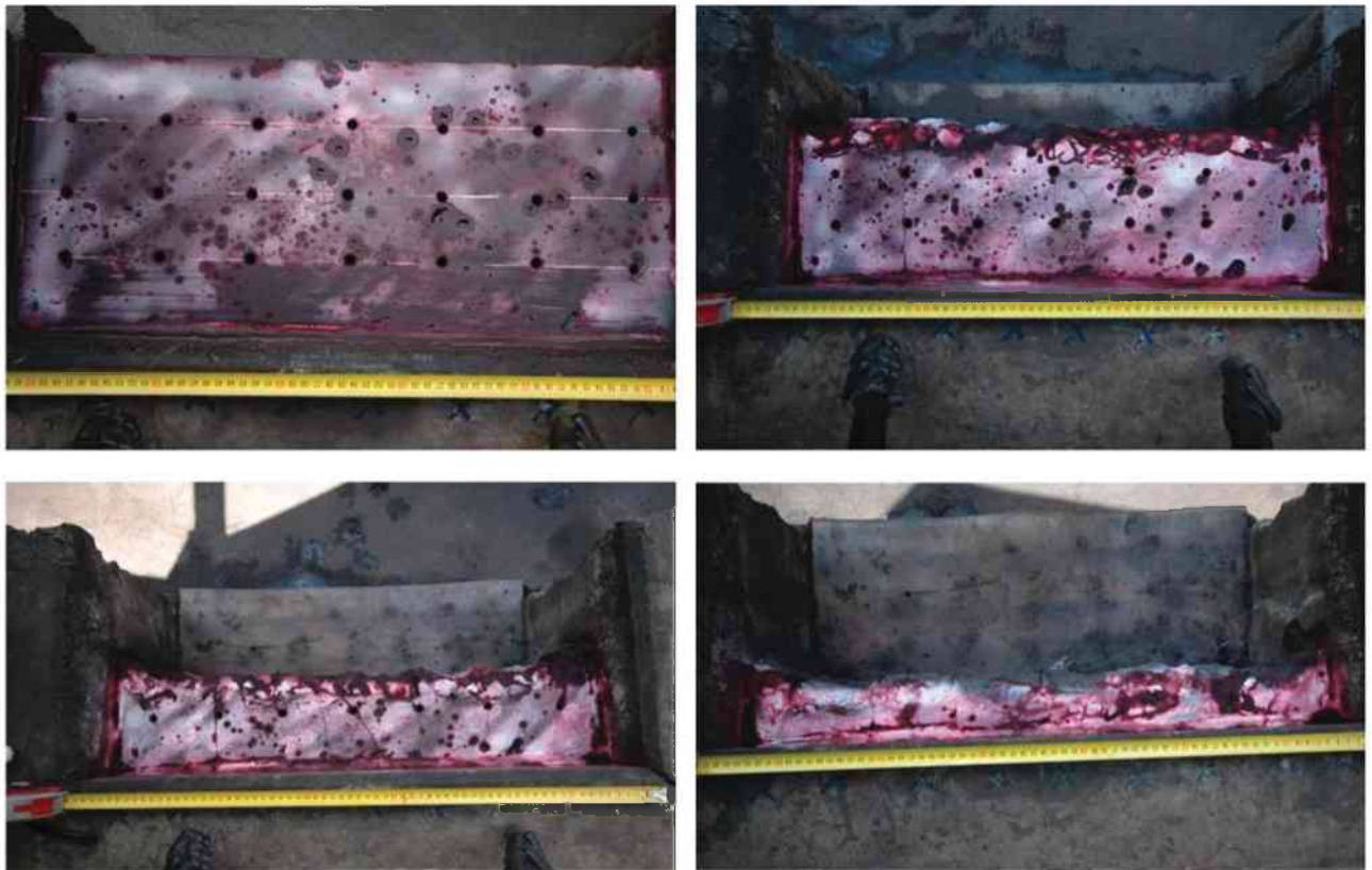
Figure 135: Crack detection on top Block B06 (Reference)
