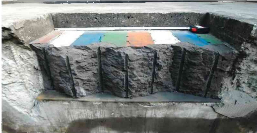
Figure 60: Front view after blasting of 1st burden deviation pattern CH01B02, row 1
