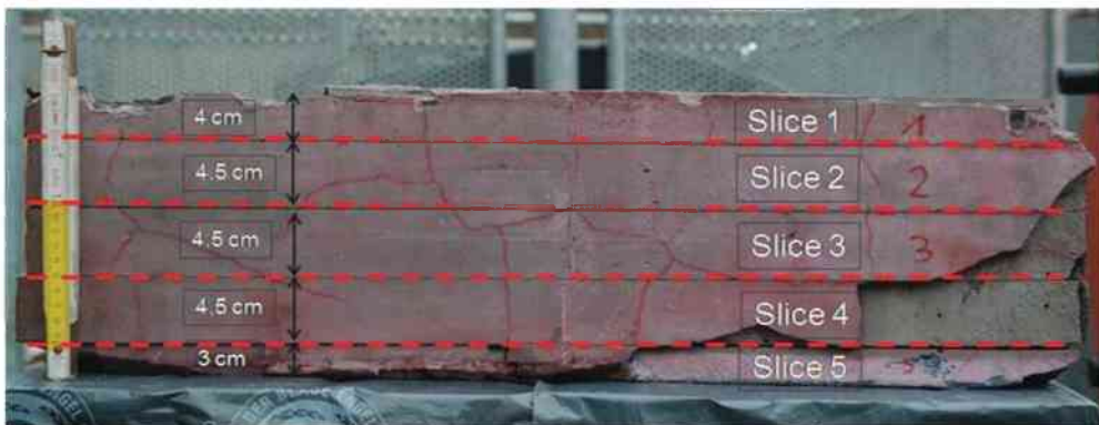
Figure 26: Distance between slices to cut the testing block CH01B04
