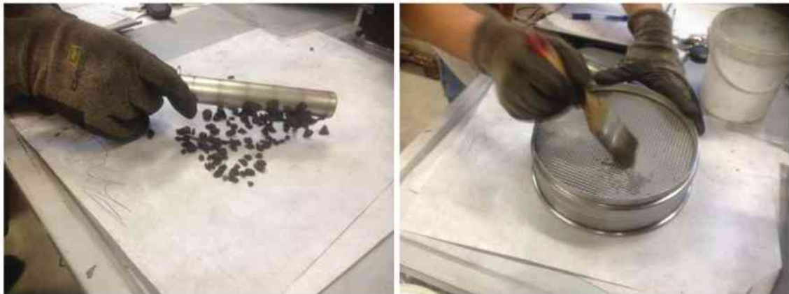
Figure 23: Magnetic separation and brush cleaning of particles remaining on the mesh cloth
