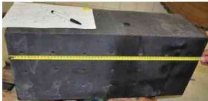
Figure 12: Testing block with dimensions 660×280×210 mm
