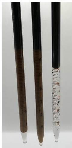
Figure 41: Phase behavior results after 204 days, a) to the right a 7500-sodium carbonate + 9 TH oil, in the middle 7500-potassium carbonate + 9 TH oil, to the right 8/9 TH softened brine + 9 TH oil.
