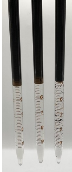
Figure 42: Phase behavior results after 204 days, a) to the right a 7500-sodium carbonate + 9 TH oil + 1900 SNF 3630S, in the middle 7500-potassium carbonate + 9 TH oil + 1850 KA 5265, to the right 8/9 TH softened brine + 9 TH oil.
