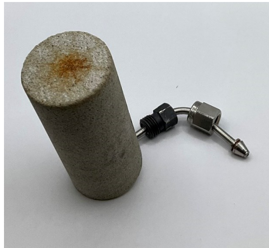
Figure 46: core plug showing corrosion on one of its faces.
